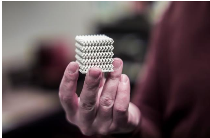
Figure 1. A 3D-printed cell structure using ceramic Vat Photopolymerization (VPP) technique. Picture by Jonne Renvall/ Ceramic Materials research group/Tampere University.
